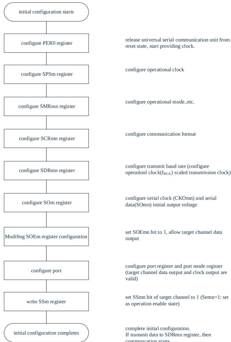
Figure 12-21: Initial set-up steps for master transmission and reception
