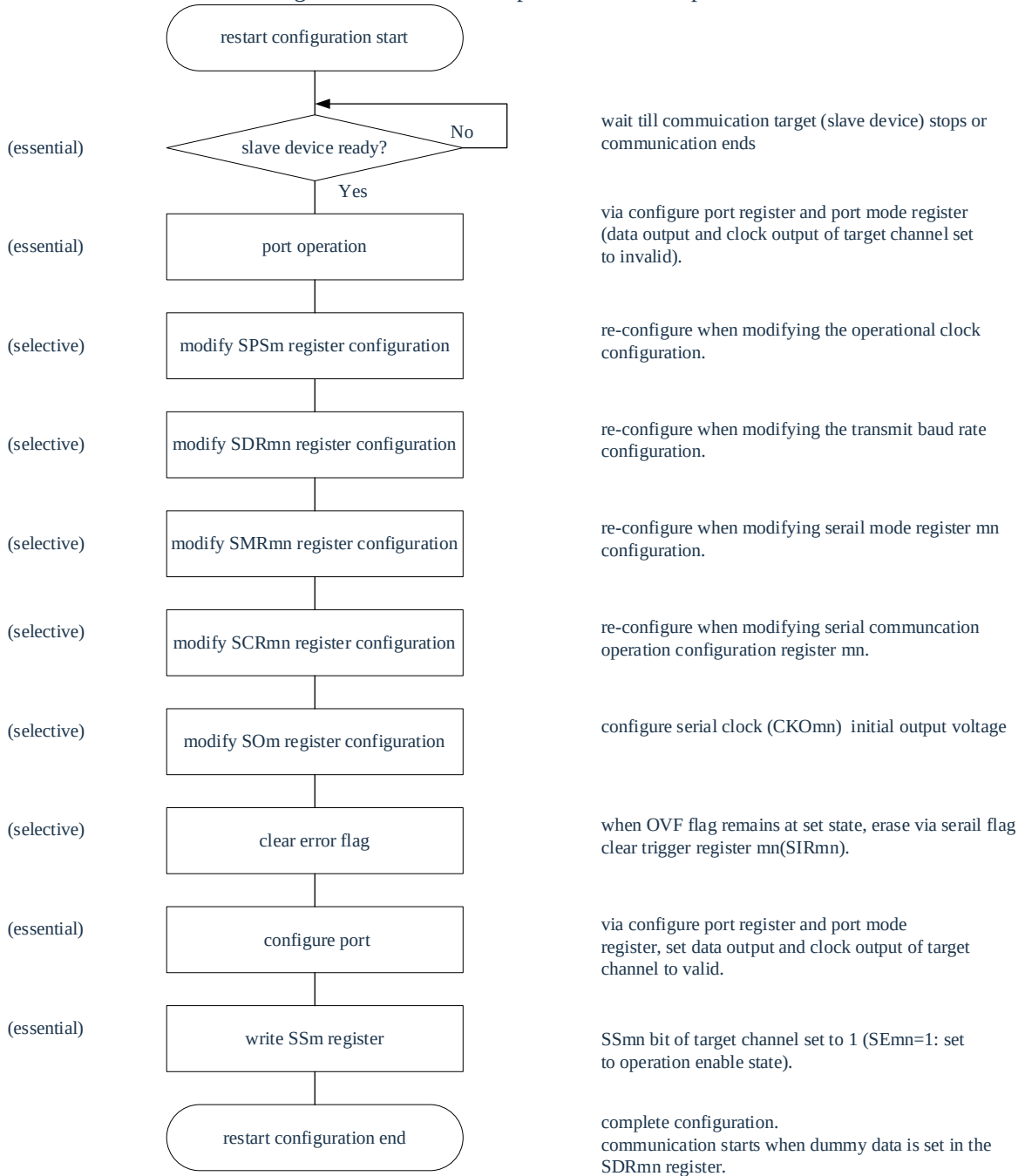
Figure 12-15: Restart steps for master reception
