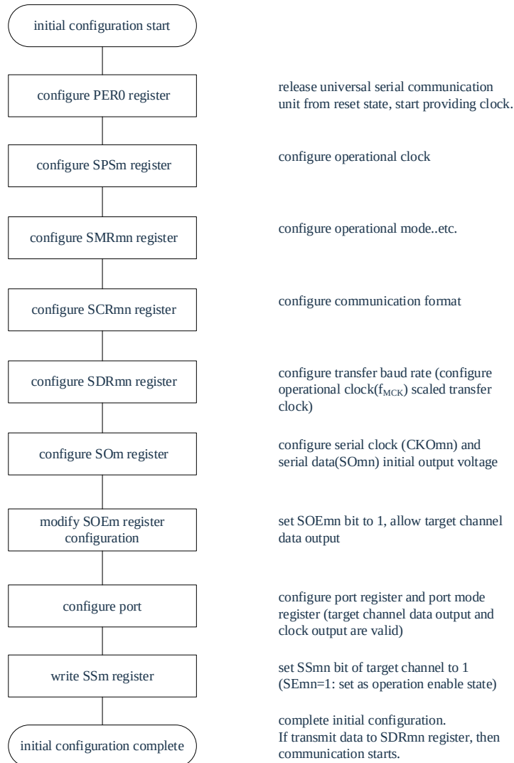
Figure 12-5: Initial setup steps for master transmission
